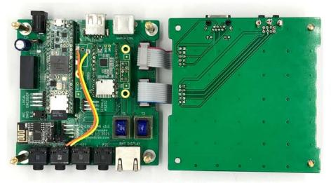
Figure 8 — A close-up of the HMI and the RJ45 port adapter boards.
