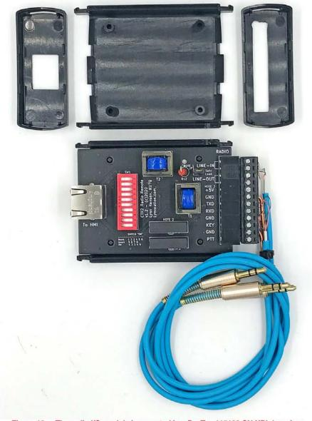
Figure 10 — The radio I/O module is mounted in a PacTec 115129 CN-XRL housing.
