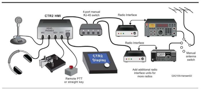
Figure 2 — A functional drawing of the basic CTR2 system.
