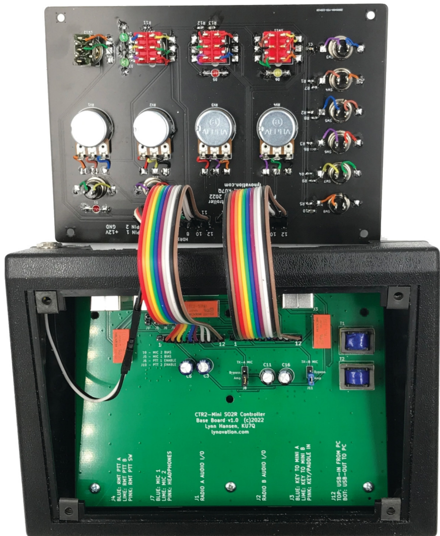
Figure 8 — Completed project showing the wiring interconnections between the front panel board and the main controller board.
