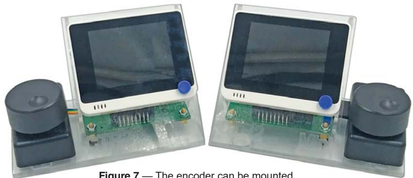
Figure 7 — The encoder can be mounted to the left or right of the display.
