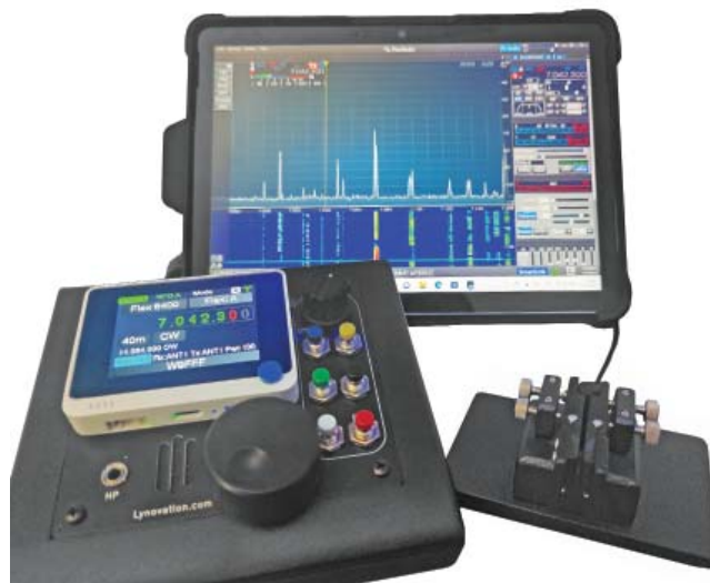
Figure 8 — A simple solution that utilizes the CTR2-Mini+, a tablet, and an iambic paddle for remote CW use. Not pictured are headphones that plug into the HP port.
