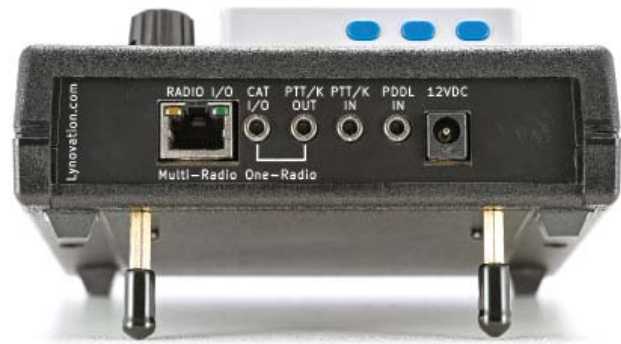
Figure 7 — The CTR2-Mini+ back panel has connections for footswitches, paddles, 12 V dc input, CAT cables, and multi-radio links.
