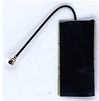
Antenna with tape installed
