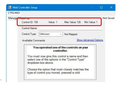
In this example I turned encoder when the *MIDI* was set to the Home encoder mode so it is controlling **Change Control (CC) 100**.
