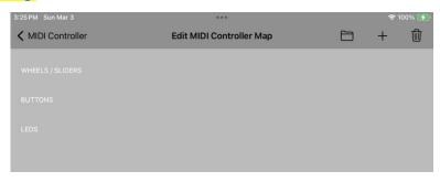
Next, turn the encoder to register the primary event of the current encoder mode in the **Wheels/Sliders** list. Once this is done, press and turn the encoder to register the secondary event. Next, short-press the encoder to move to the next encoder mode (yellow LEDs will change) and register its primary and secondary events. Continue this process until you have registered all four encoder modes for a total of 8 slider controls.
