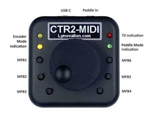
The green LED flashes once every 2 seconds when the unit is first powered up. It changes to two flashes every second when the unit is connected via Bluetooth-LE to the app.
