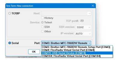
Since you are connecting to a USB serial port there is no need to set the baud rate. It will run at USB speed regardless of the baud setting.
