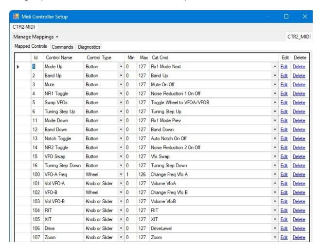
**NOTE:** Make sure you run the encoder to the full CCW and CW directions so the minimum and maximum values are recorded. This is especially important on **Slider** controls that have the full range from 0 to 127 counts.
