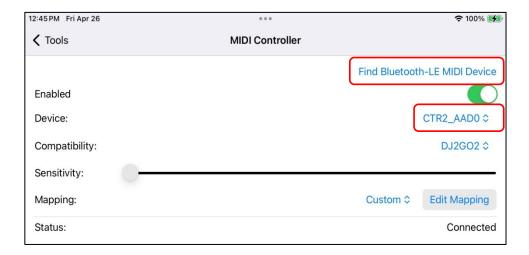
If CTR2\_xxxx does not appear on the Device list, or it doesn't connect when turning the Enabled switch On press the Find Bluetooth-LE MIDI Device button again. You may need to press this button several
