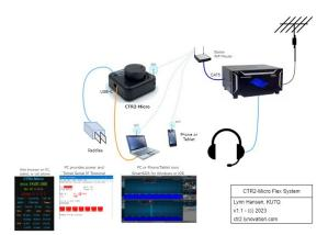
NOTE: You can't use the hotspot on your tablet, cell phone, or a StarLink connection to connect your Micro to a remote Flex radio even with a VPN because these systems use Carrier Grade Network Address Translation (CGNAT) that blocks port forwarding.
