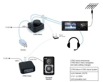
It can also be set up as a WiFi access point. This eliminates the need for an external router. The Micro connects directly to **CTR2**-**Voice** using SSID *CTR2-Voice* and password *ctr2-voice*. Set the **CTR2-Voice** IP address in the **Configure -> Report** menu to *192.168.4.1* and unmute the report.
