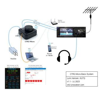
A serial terminal program runs on the station computer and provides a display to configure the Micro for your needs. Once the WiFi link is configured you can use a network based <u>Telnet terminal program</u> or a <u>web browser</u> on your cell phone or tablet to view and control the Micro.
