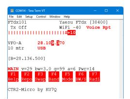
If your radio supports reading the S-meter over CAT an S-meter graph will be displayed on the second line of the Home page. In this example the S-meter is reading 10dB over S9. The S-meter is not supported in the browser.
