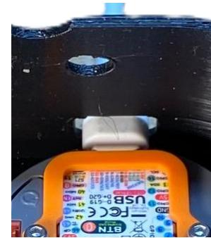
**WARNING:** The ring nut should be finger tight. Do not overtighten it! This will cause additional friction on the gray ring on the M5Dial, making it harder to turn.
