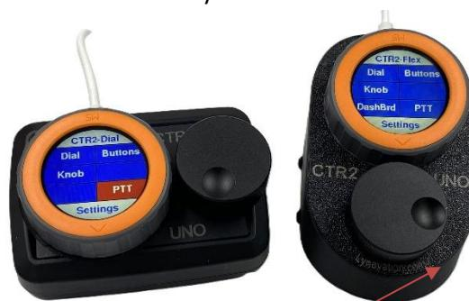
The **Duo's** hardware is similar to the **Duo** and **Quad** in that it provides a physical knob, and supports CW paddle, straight-key, and PTT inputs. It also provides a speaker with a **volume control** to provide a useable sidetone for CW operation when running **CTR2-Flex** firmware.
